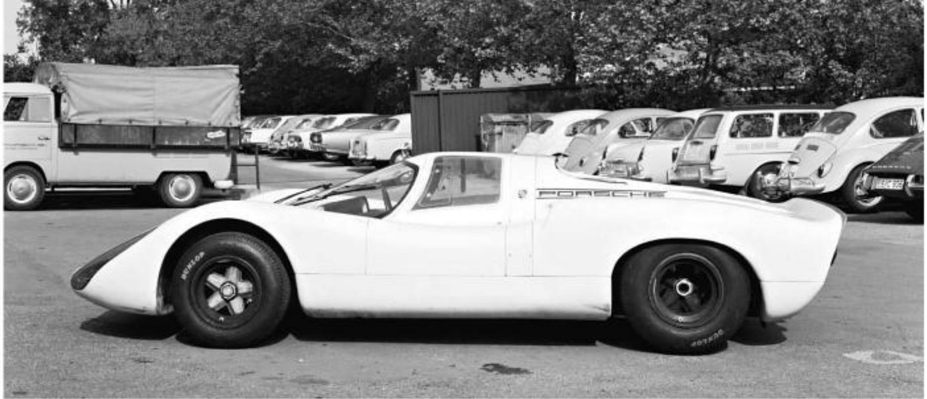
Conversion: The first 908 short-tail coupés differed from the 907 in body details as a result of installation of the three-liter, eight-cylinder engine.
