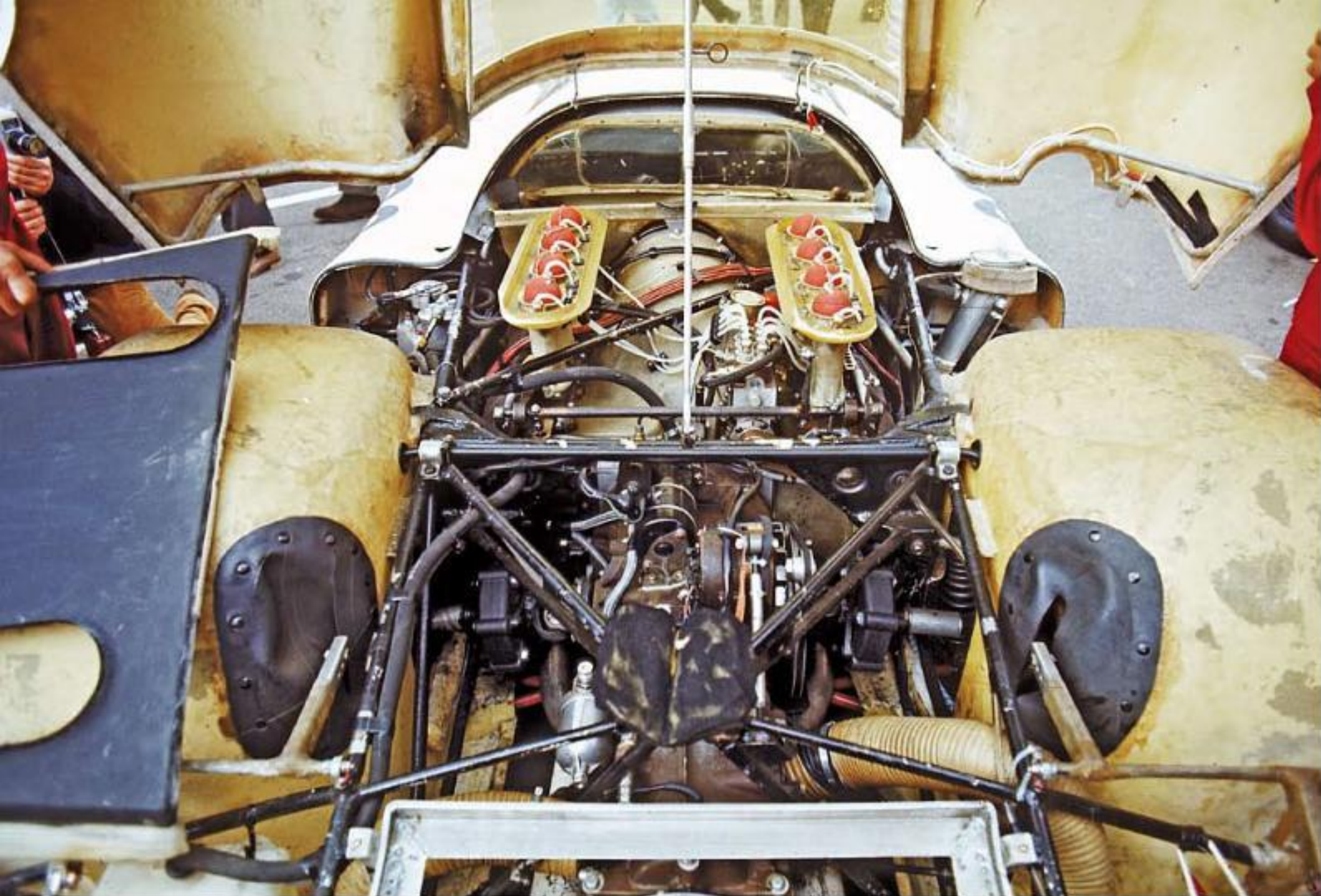
Flexible: Even in its first outing at the Le Mans practice in April 1968 the three-liter showed its potential. Despite its modest 335 horsepower, the engine was quite driveable and produced usable power between 5500 and 8500rpm.
