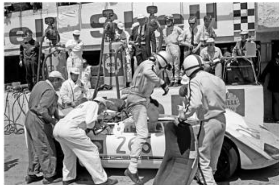
Custom tailored: Mitter and Schütz trade places behind the wheel of the winning 908/02. A driver change includes swapping the racing seat; each driver has his own personal racing bucket seat.
