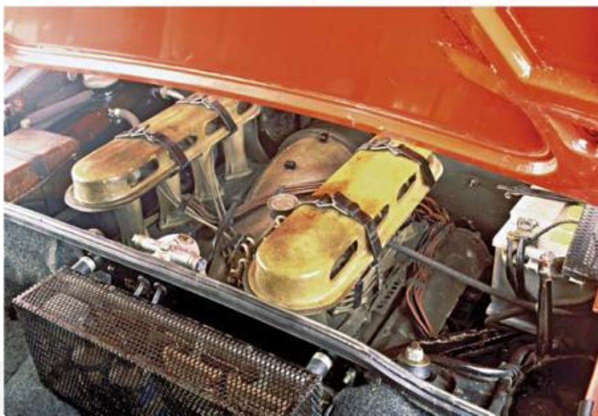
Plenty of room in the back: The compact three-liter engine was a perfect fit in the 914.
