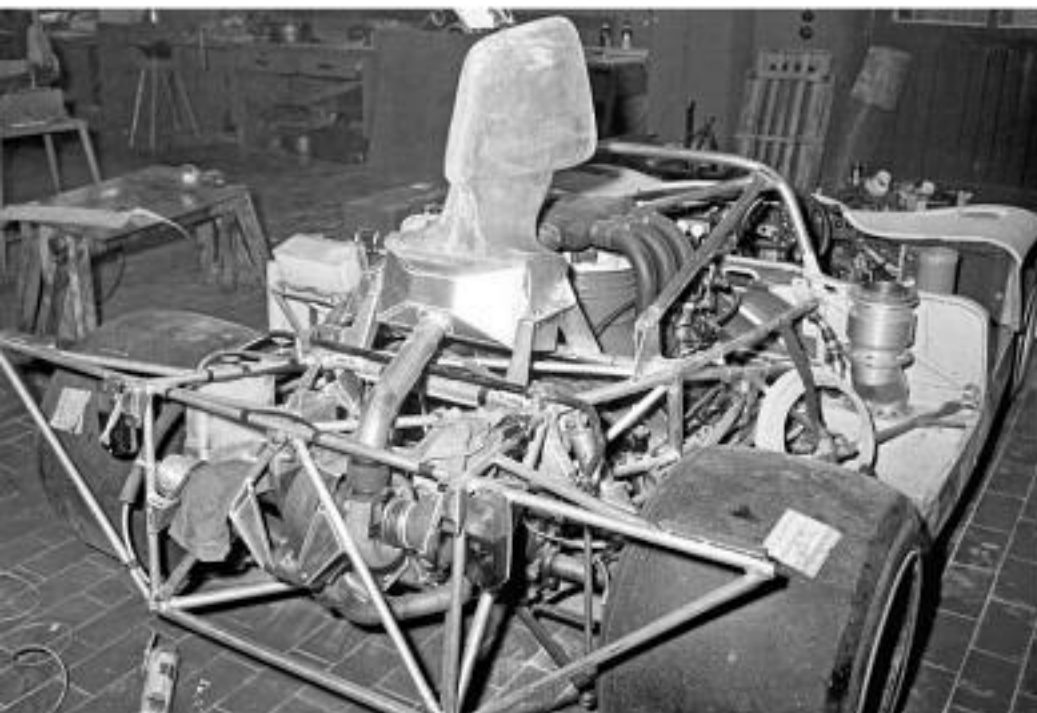
Cage raised: From 1975 onward, the delicate latticework of the /03 contained an impressive 500 turbocharged horses.
