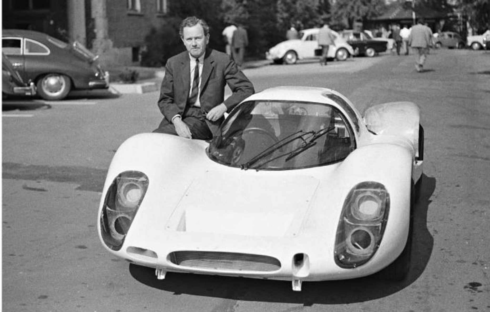
Porsche on Porsche: In 1968, Ferry Porsche, son of the company founder, poses on the 908 coupé, which is still missing its rear bodywork. The first examples of the 908/01 (the /01 designation was applied retroactively, once there was an /02) may be identified by the vertical opening on the port side of the nose.
